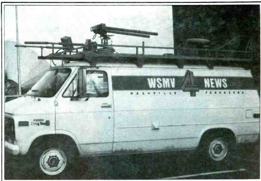
A typical television remote telecast unit. It communicates with the studio on 450.55 MHz. Barrel-shaped objects on roof are used for microwave transmission of video.
