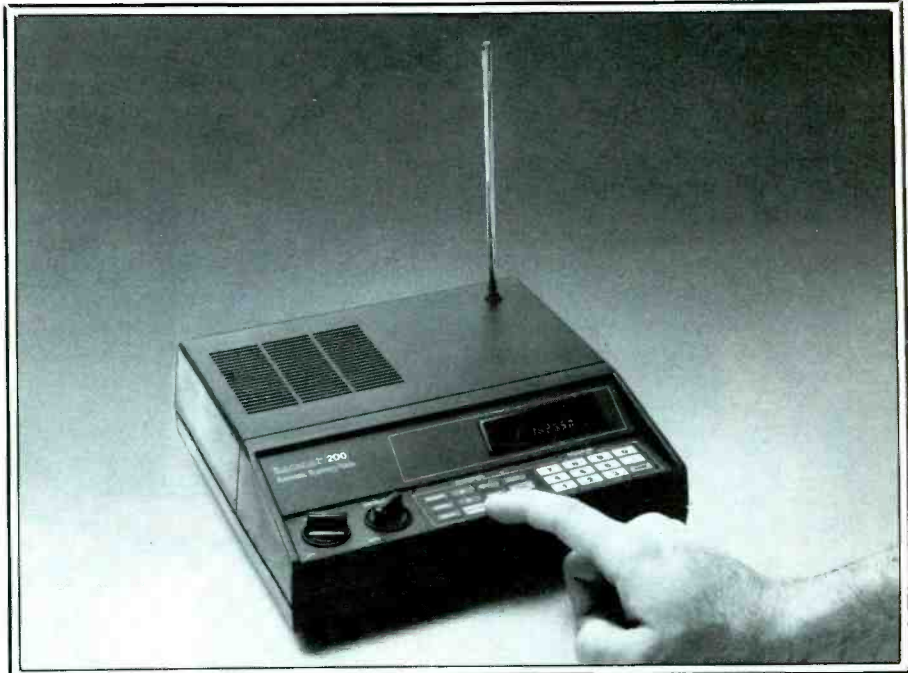
Some scanners, such as this Bearcat 200, offer direct access to weather channels, which would be helpful during a weather emergency.
