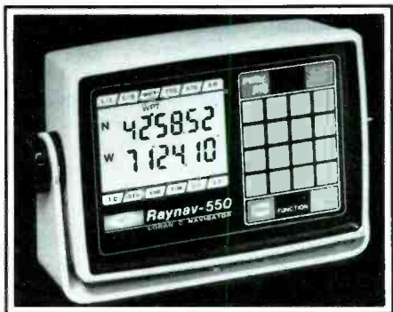
Raytheon's RAYNAV-550 Loran C Navigator.
