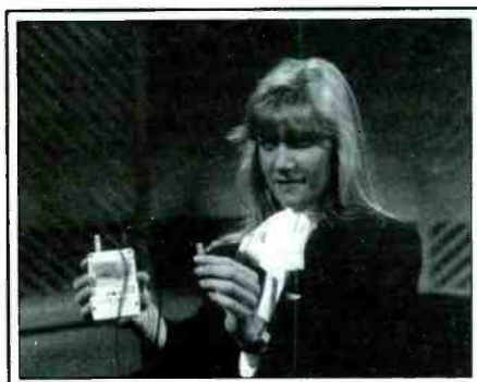
This wireless microphone transmits on 174.80 MHz. The transmitter attaches to the users belt and the tiny microphone clips on necktie or shirt collar.
