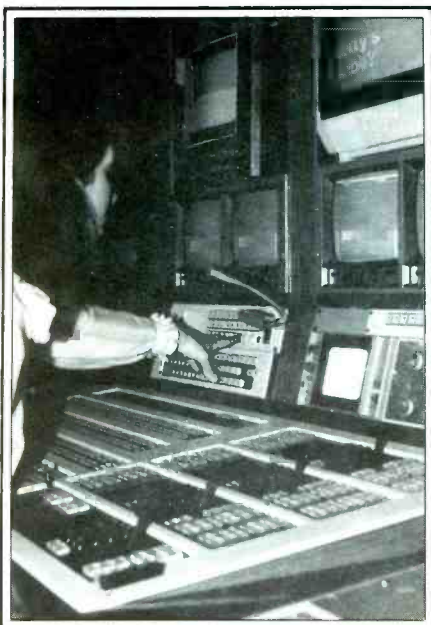
Studio control room director gives standby cue to a remote telecast unit. This systems uses a 450.85 MHz radio link.
